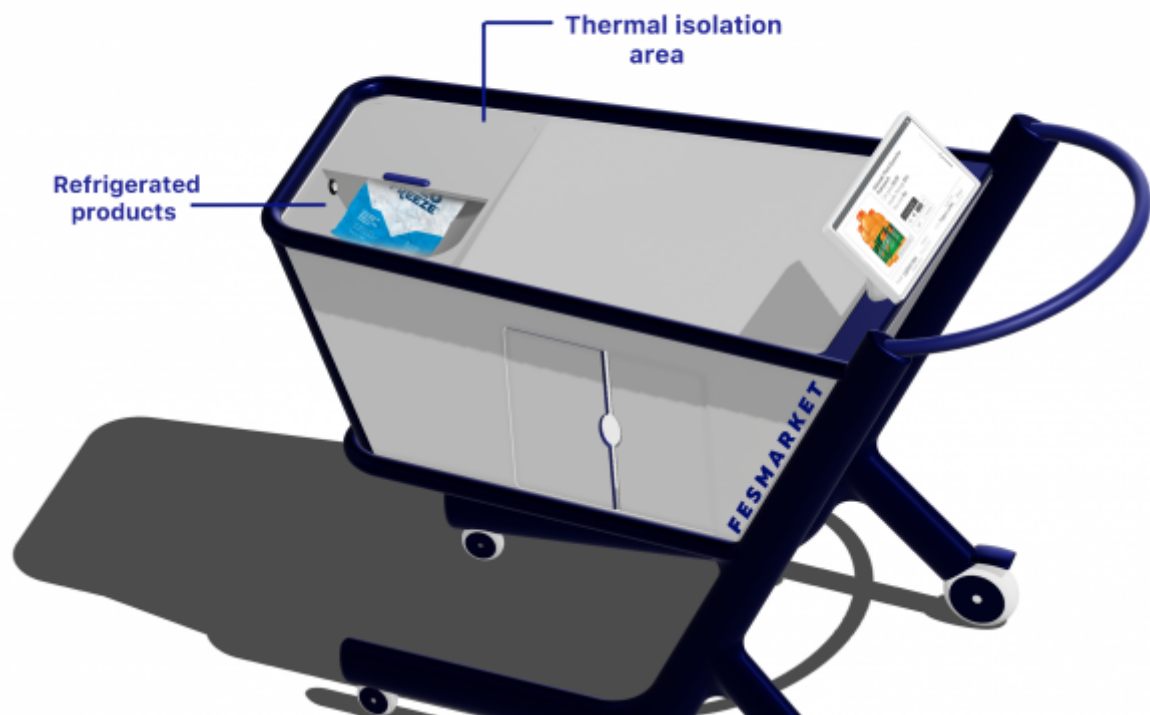
Figure 65: Thermal isolation view
